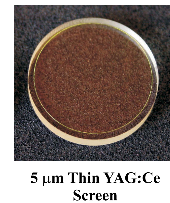
Thin YAG:Ce Screen on FOP
