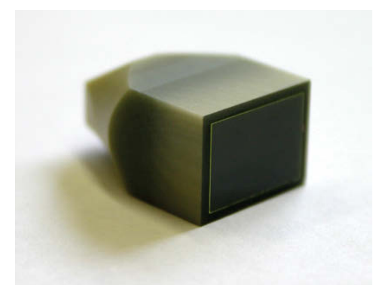
Thin YAG:Ce Screen on FOP
